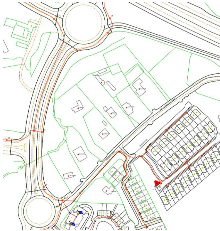
Existing Virgin Media Infrastructure
